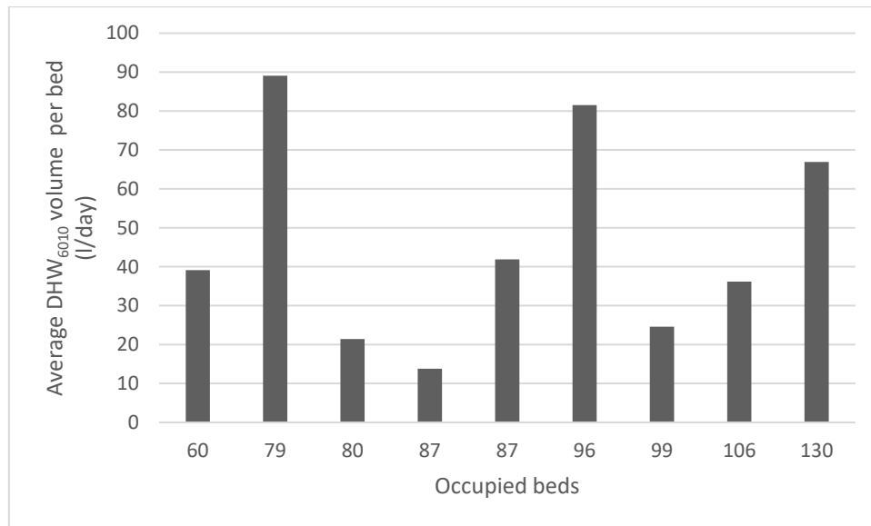
Figure 1 - Average hot water volume per bed, with respect to the number of occupied beds
