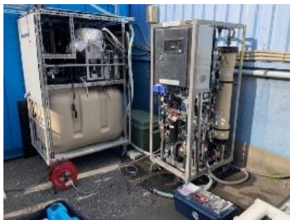
Figure 5-Raw water tank, filtration device / water purification device
